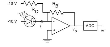
Photodiode current at minimum irradiance:  $i_{\min} = H_t(E_{\min}) = 4.112 \,\mu\text{A}$ .  $E_{\max} = \frac{x_{\max}}{r^2} = 3.880 \,\frac{\text{mW}}{\text{cm}^2}$  and  $i_{\max} = H_t(E_{\max}) = 8.225 \,\mu\text{A}$ . At  $x = 10 \,\frac{\text{W}}{\text{sr}}$  want  $v_o = 0 \,\text{V}$ , so find  $R_{\text{C}}$  that satisfies:
