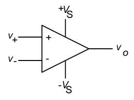
Here,  $v_{+}$  and  $v_{-}$  are inputs.
