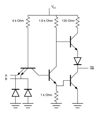
Input to gate is a transistor emitter.
