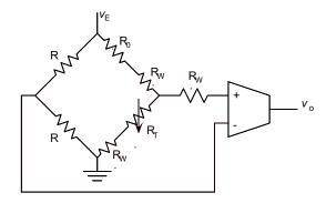
$R_{\mathrm{w}}$  is resistance of wire. Output,  $v_o$ , should not be a function of this.
