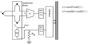
Instrumentation Amplifier Gain
