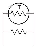
Transfer function:  $H_{t3}(x) = \frac{R_{\rm M}}{2} \left( 1 + \frac{\alpha}{2} \Delta x \right),$
