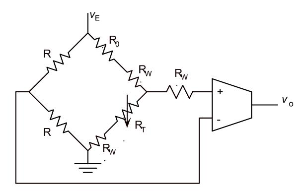
$R_{\rm w}$  is resistance of wire. Output,  $v_o$ , should not be a function of this. Re-write RTD function as  $H_{\rm t}(x) = R_0 + R_0 H'_{\rm t}(x)$ , where  $H'_{\rm t}(x) = \alpha_1 x + \alpha_2 x^2$ .
