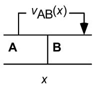
Potential developed,  $v_{AB}(x)$ , a function of metals and temperature.
