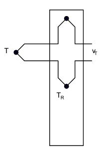
Block upon which connections to thermocouple leads are made.
