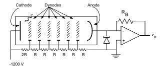
Bias to dynodes provided by a ladder of resistors, sometimes called a bleeder circuit.
