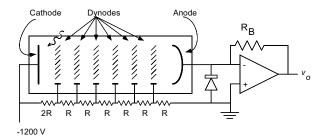
At least three plates in an evacuated tube, one plate exposed to light.
