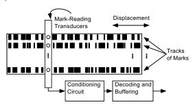
A strip or disk of some material, such as plastic, is mounted on object or on something linked to the object.
