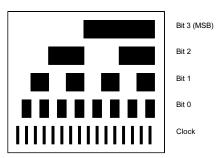
For an n-bit precision device, n+1 tracks or rings are used.
