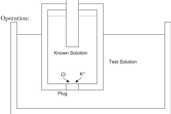
A small amount of ions can flow through the plug.
