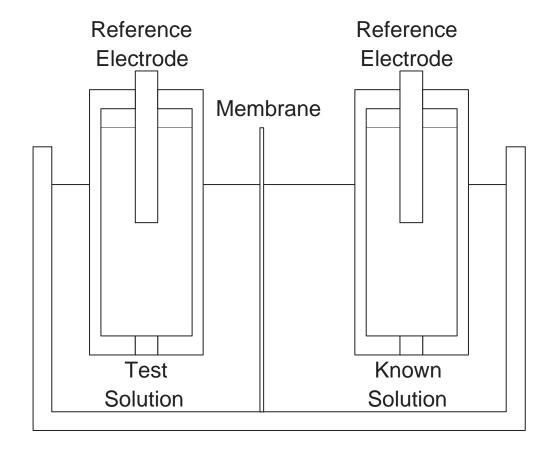
Test ions cross membrane, causing a potential to develop across the membrane.
