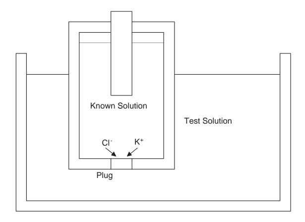
A reversible electrode is placed in a small container with a solution of known concentration.
