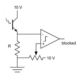
Choose phototransistor with response,  $H_{t2}(x) = xK_s$ , where  $K_s = 300 \frac{\mu \text{A cm}^2}{\text{mW}}$ .
