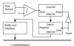
Flow sensor generates a voltage pulse train.
