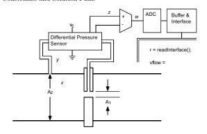
• Choose orifice diameter so that differential pressure is in range  $[0, p_{\text{max}}]$ :
