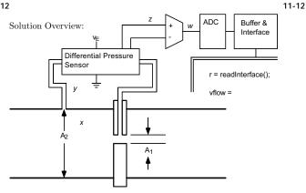
$\bullet$  Use an orifice plate flow transducer. Call area of orifice  $A_1$ . Call response and output of flow transducer
