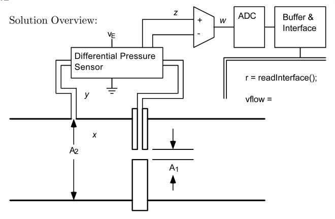
• Use an orifice plate flow transducer. Call area of orifice  $A_1$ .
