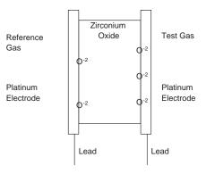
Consists of zirconium oxide,  ${\rm ZrO}_2$ , between platinum electrodes.
