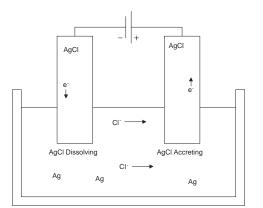
In forward direction current flows from electrode to solution (electrons flow from solution to electrode).
