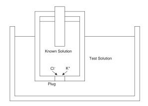
A reversible electrode is placed in a small container with a solution of known concentration.
