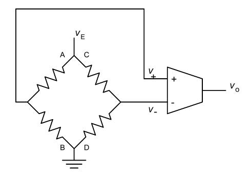
Arm A:  $H_{t2}(x) = R - R_s = R(1 - xk).$ Arm B:  $H_{t1}(x) = R + R_s = R(1 + xk).$ Other Arms: Resistor of value R.
