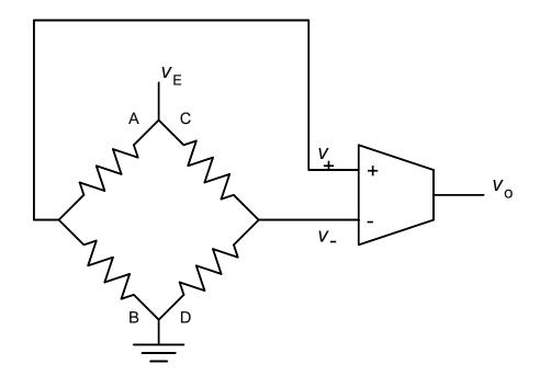
Arms A and D:  $H_{t2}(x) = R - R_s = R(1 - xk).$ Arms B and C:  $H_{t1}(x) = R + R_s = R(1 + xk).$
