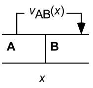
Potential developed,  $v_{AB}(x)$ , a function of metals and temperature.
