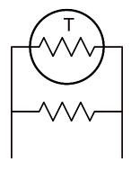
Transfer function:  $H_{t3}(x) = \frac{R_M}{2} \left( 1 + \frac{\alpha}{2} \Delta x \right),$
