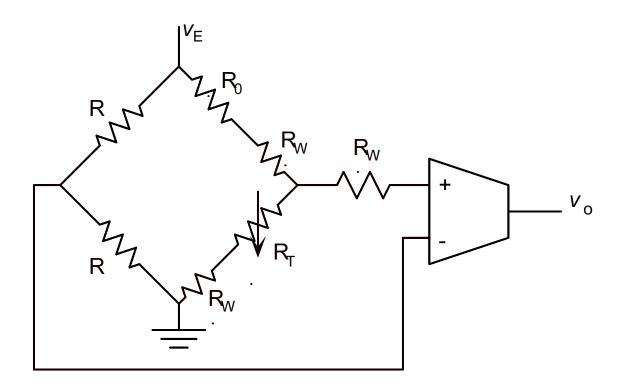
$R_{\rm w}$  is resistance of wire. Output,  $v_o$ , should not be a function of this. Re-write RTD function as  $H_{\rm t}(x) = R_0 + R_0 H'_{\rm t}(x)$ , where  $H'_{\rm t}(x) = \alpha_1 x + \alpha_2 x^2$ .
