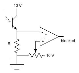
Choose phototransistor with response,  $H_{t2}(x) = xK_s$ , where  $K_s = 300 \frac{\mu \text{A cm}^2}{\text{mW}}$ .
