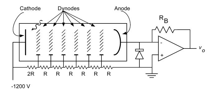
Bias to dynodes provided by a ladder of resistors, sometimes called a bleeder circuit.
