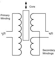
A three-winding transformer with a movable core.
