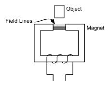
Consists of a coil of wire wrapped around a c-shaped magnetic core.
