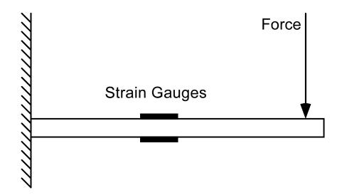
The upper part of beam is stretched (positive strain) ... ... and the lower part of beam is compressed (negative strain).
