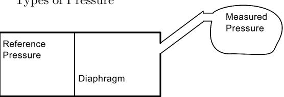
This can be visualized as the pressure on a diaphragm, with the pressure being measured on one side and the reference pressure on the other.
