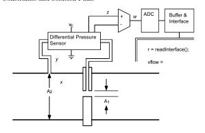
• Choose orifice diameter so that differential pressure is in range [0,  $p_{\rm max}$ ]:
