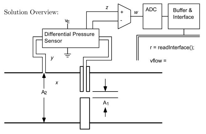
$\bullet$  Use an orifice plate flow transducer. Call area of orifice  $A_1$ .
