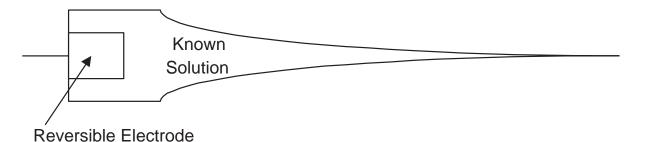
Reference electrode container in shape of tapered tube.
