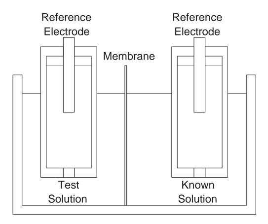
Consists of a container divided into two halves by a membrane.
