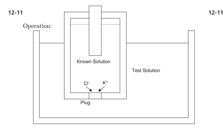
A small amount of ions can flow through the plug.
