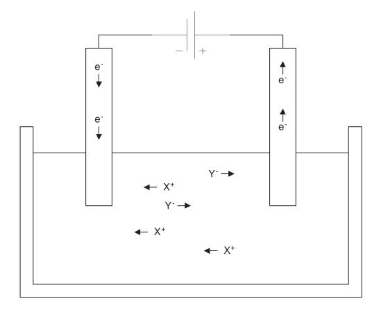
Current flow in metal is by the motion of electrons, as usual.
