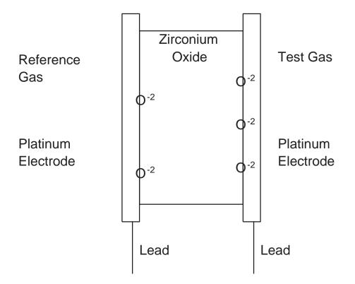
Consists of zirconium oxide, ZrO<sub>2</sub>, between platinum electrodes.
