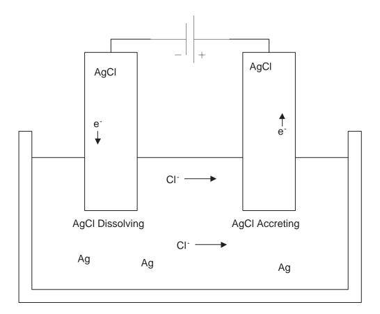
In forward direction current flows from electrode to solution (electrons flow from solution to electrode).
