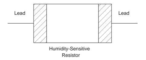
Transducer consists of leads placed on a special material.
