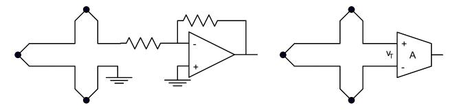
The differential inputs to the instrumentation amplifier cancel noise, this noise is not canceled with the single input used in the inverting amplifier.
