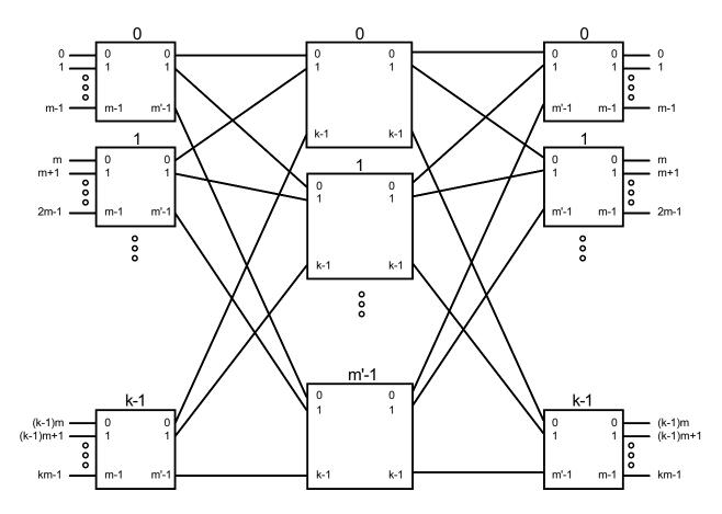
Topology of Clos network in which  $m' > (m-1)(x+d^{1/x})$ ,
